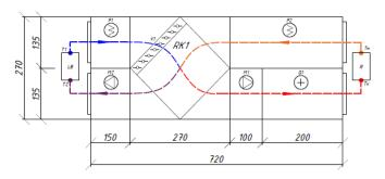
Figure 1: General view of the experimental system: RK1–investigated plate air-heating recuperator; F1– Supply filter; F2–exhaust filter; M1–Supply fan; M2–Exhaust fan; Q1–electric calorifier; T1 and T2– temperatures of the supply and exhaust air; Тк–air temperature in the heated room; Тн–temperature of the exhaust air from the room; V1–an adjustable damper.
