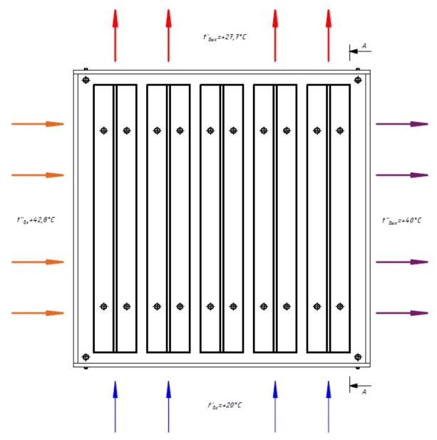
Figure 2: Diagram of the air flows movement in the investigated plate air-heating recuperator
